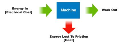
The same is true for diesel fuel powered tasks. Part of the fuel is consumed in overcoming internal friction; the balance is actually applied to the work being done.
